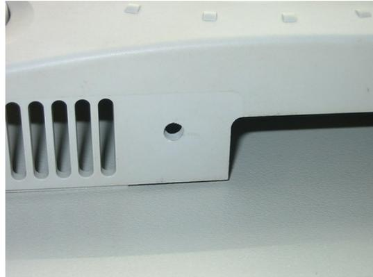
Now take your hot glue gun and warm it up. Test if the button fits and doesn't jam, so try it out a couple of times, it should make a clicking sound like usual. No worries if the hole is a little bit too wide, it's better than trying to push it in and it gets stuck...
